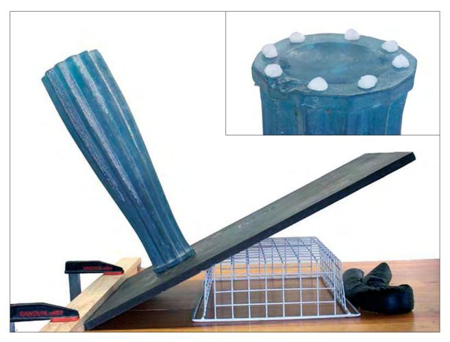
Fig. 3 (inset) Utility Wax applied to the base of a test vase (photo by Norm Heke). Fig. 4 Set-up of vase for test (photo by Norm Heke).
