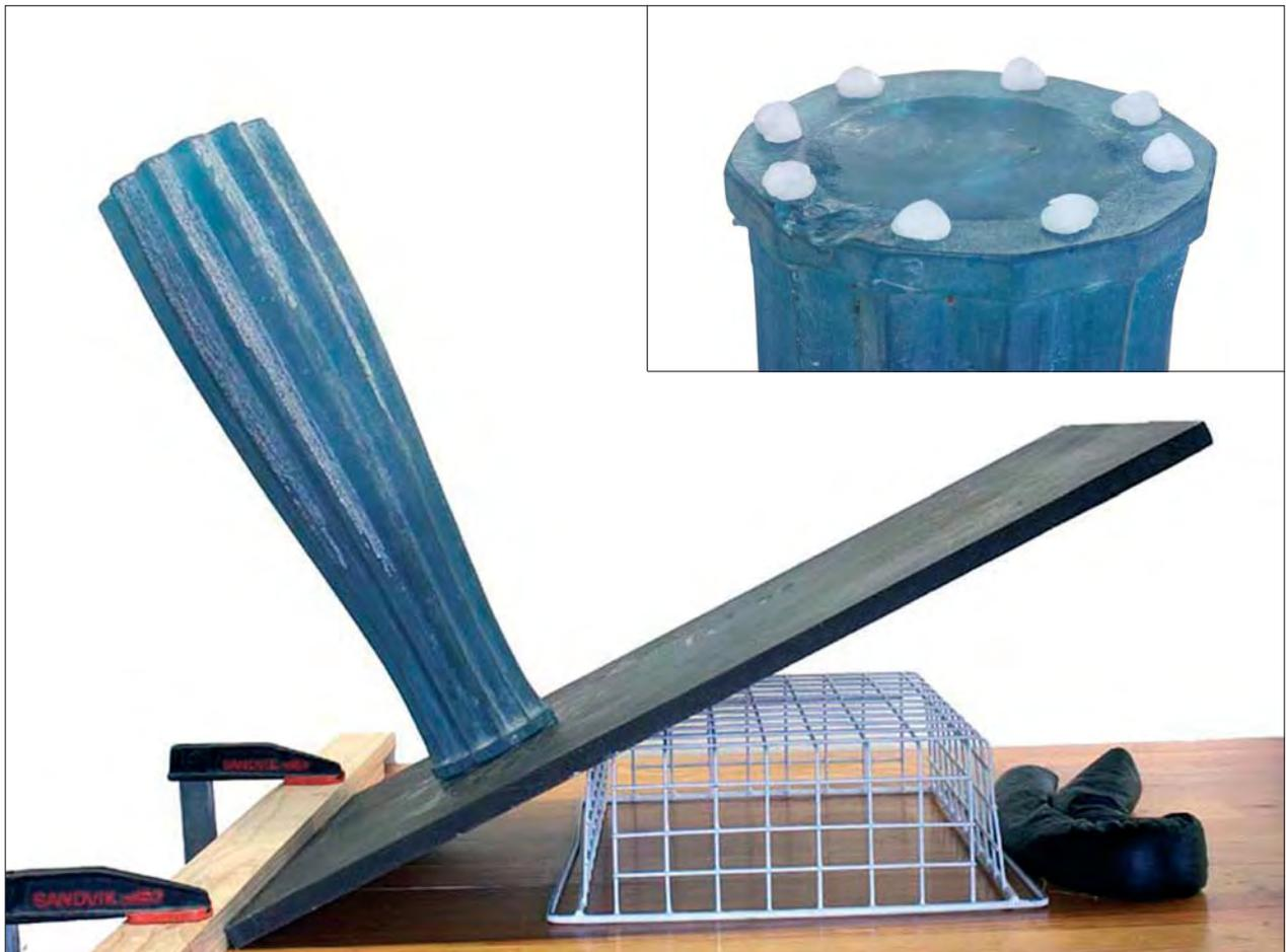
Fig. 3 (inset) Utility Wax applied to the base of a test vase (photo by Norm Heke).
