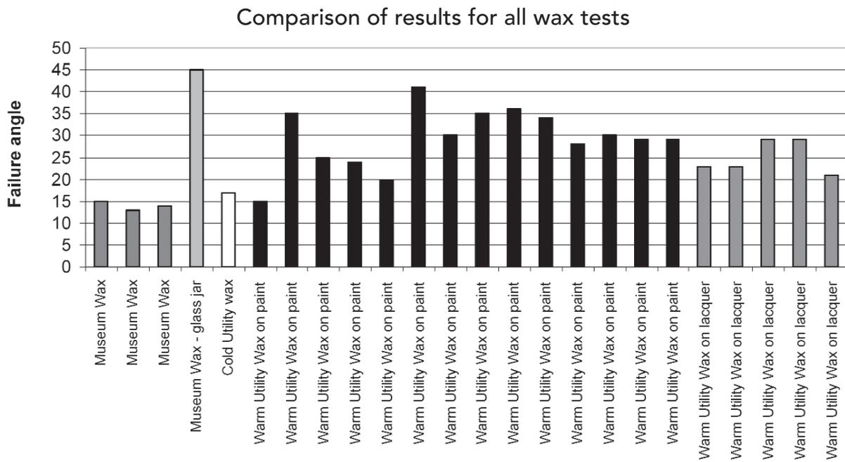
Fig. 5 Adhesion bond failure angle for all wax tests.
